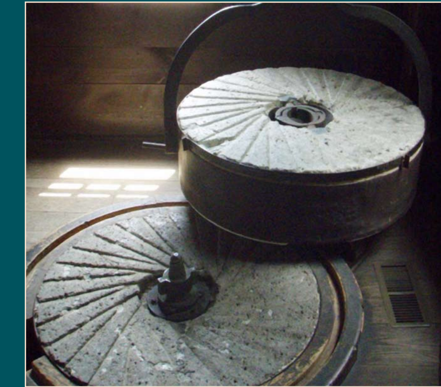
Up until 1890 most of the flour in America was made using millstones. The bottom stone was fixed to the floor, while the top stone was turned by the main shaft, driven by the waterwheel. The distance between the stones could be varied to produce the grade of flour required; moving the stones closer together produced finer flour. Photo from the Henry Ford Museum courtesy of C.A. Sheild.
